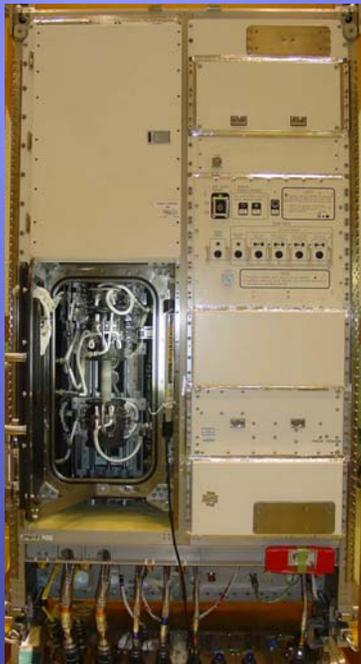
GHF is a electric furnace which generate temperature gradient on the sample to produce a single crystal alloy semi-conductor.
