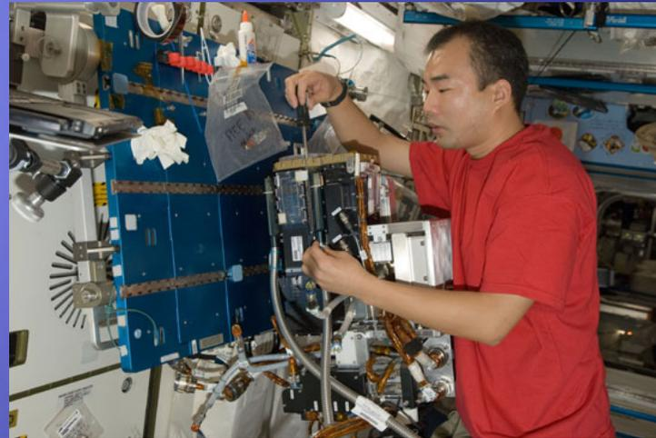
On board maintenance by astronaut Soichi NOGUCHI to fix the sealing of experiment cartridge.
