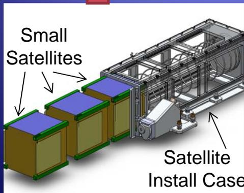
① Small satellites with Satellite Install Case.
