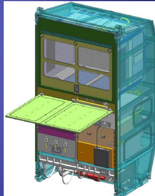
MSPR is a versatile payload rack which provides experiment space, working table, and resources such as electric power and communications for small experiment equipment.
