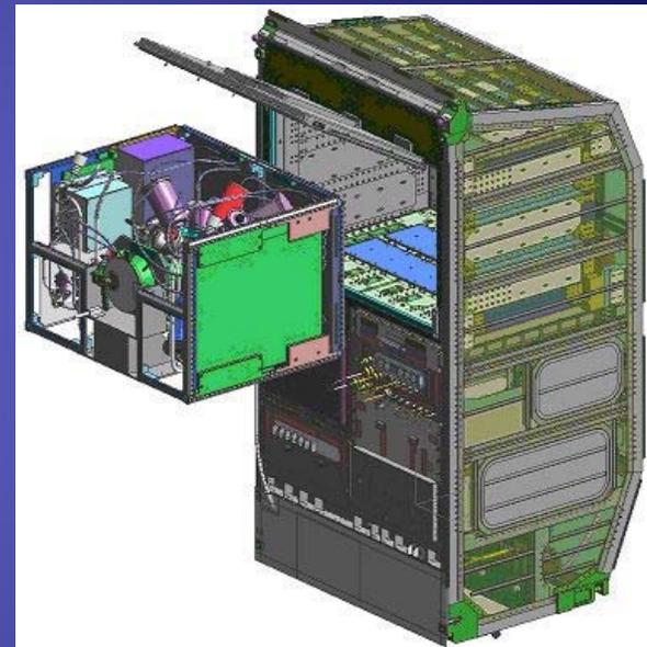
ELF measures the thermo-physical properties of fused materials such as metals and oxides. It levitates materials using electrostatic force and melt them with laser heaters to enable containerless processing in microgravity.
