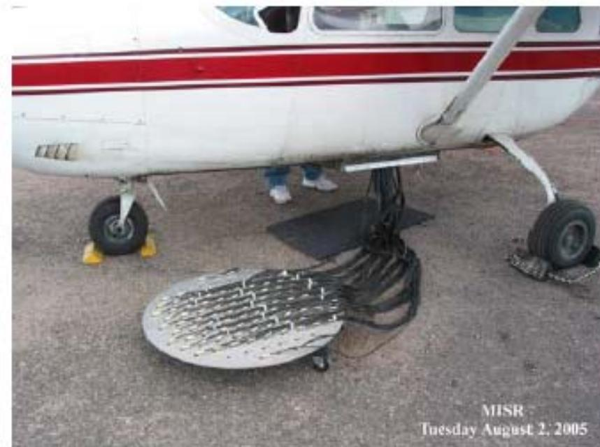
Airborne 96-element phased-array GPS antenna
