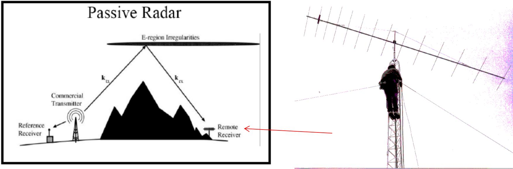
PBR for ionospheric disturbances: Reference receiver registers original signal
