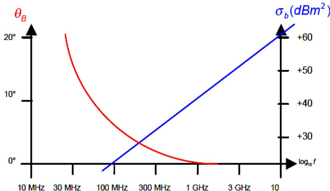
Variation of forward scatter RCS and angular width of response ( $d = 10\text{m}$ ,  $A = 10\text{m}^2$ ).
