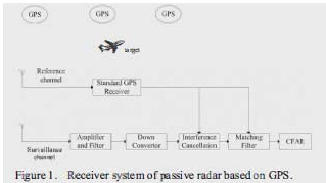
Figure 1. Receiver system of passive radar based on GPS.
