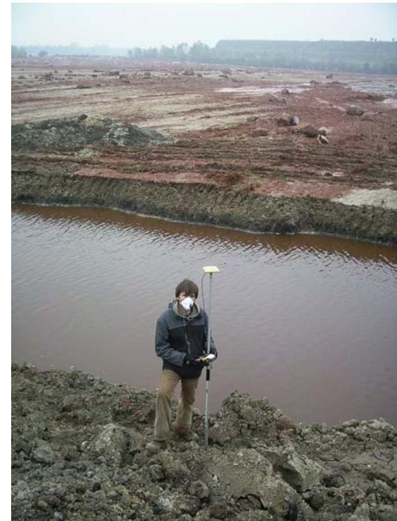
GPS technology however helped the local, on the spot event mapping and the dike deformation survey.
