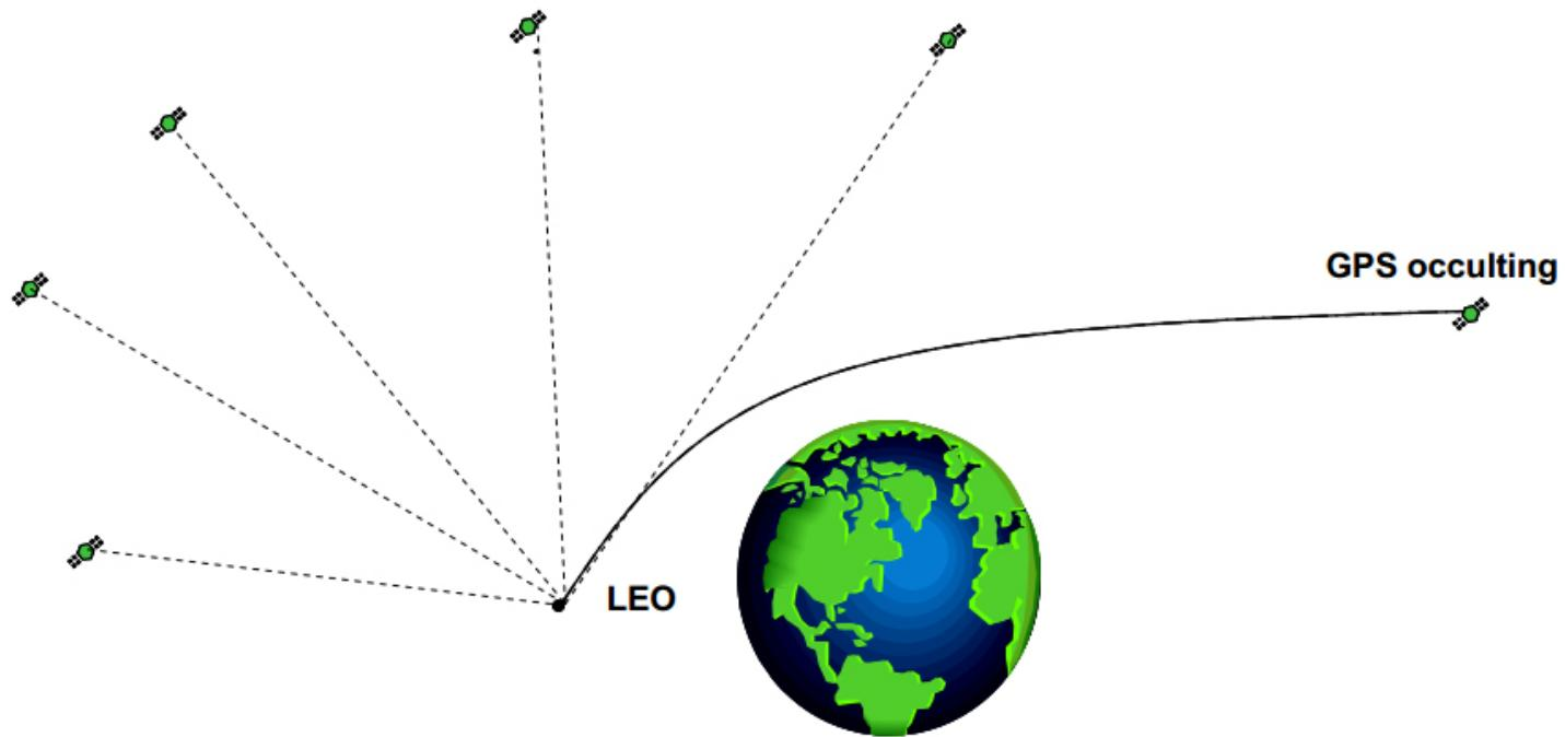
How the paths of radio signals are bent by refractive index gradients in the atmosphere and the ionosphere
