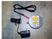
A 100 mV antenna for ionospheric signals, which is connected to the receiver.
