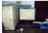
A PC to process data and provide signal strength. It is the SuperSID receiver software interface. SuperSID is the software.
