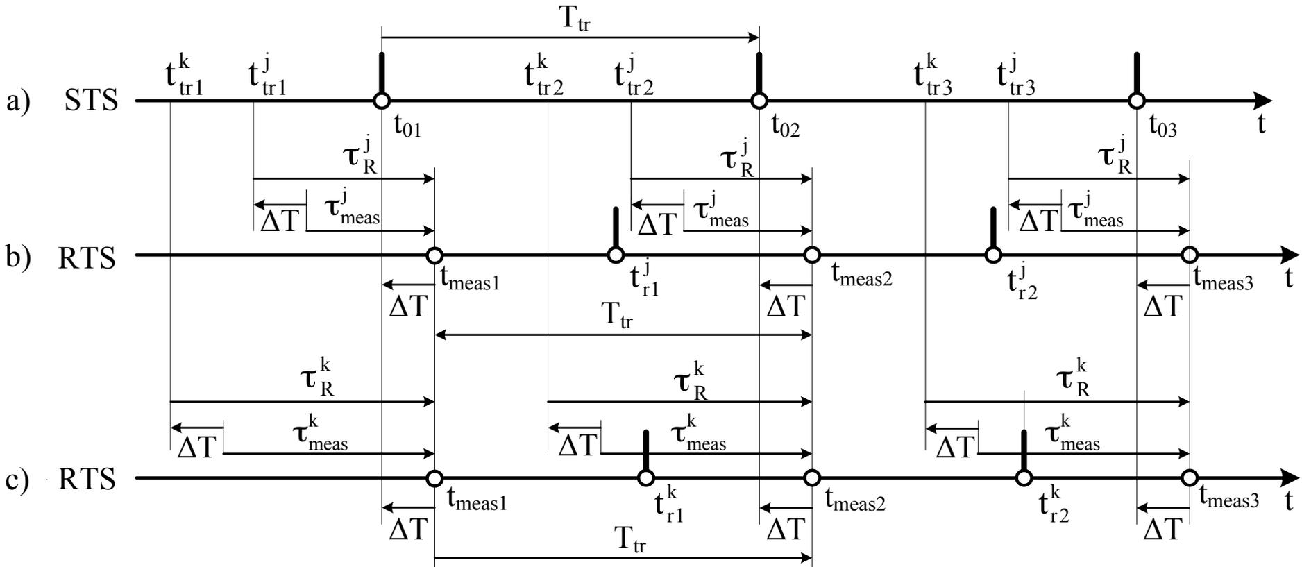
Measurement moment  $t_{meas}$  and appropriate for it transmission times for  $j$ -th  $t_{tr}^j$  and  $k$ -th  $t_{tr}^k$  satellites.
