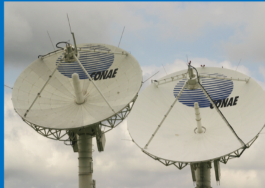
Antennas of 7 y13 m for TT&C of EO missions.
