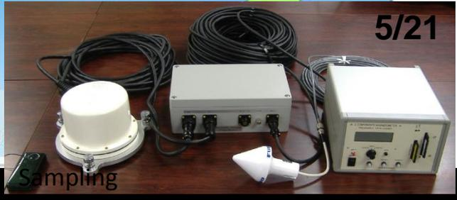
Sampling  $\Delta T=10\text{Hz}$  MAG-9 MAGNETOMETER
