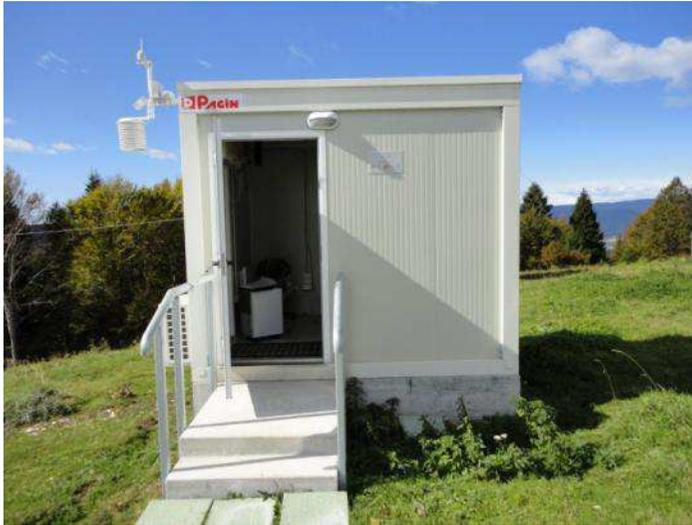
The BU camera is lodged in a small container, which has been equipped with temperature and humidity controls, and safety devices. Two telescopes can be sited inside the container. The glassy domes are permanently open. Only occasional maintenance operations are required by the Observatory technical staff.
