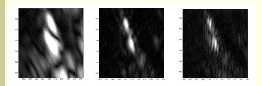
Two buildings on radar image. Left- VHF-band radar image, center- P-band radar image, VHF+P band radar image
