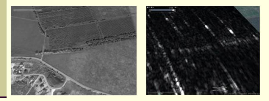
Forest landing RADAR (right), optical equipment (left), bandwidth 30 MHz, radiation mode CHIRP pulses step 5 m pixel.
