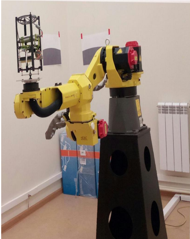
The nanosatellite, mounted on manipulator
