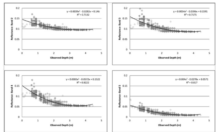
Fig1: Relation between Landsat-8- LDCM bands reflectance and lake depth measured in the field
