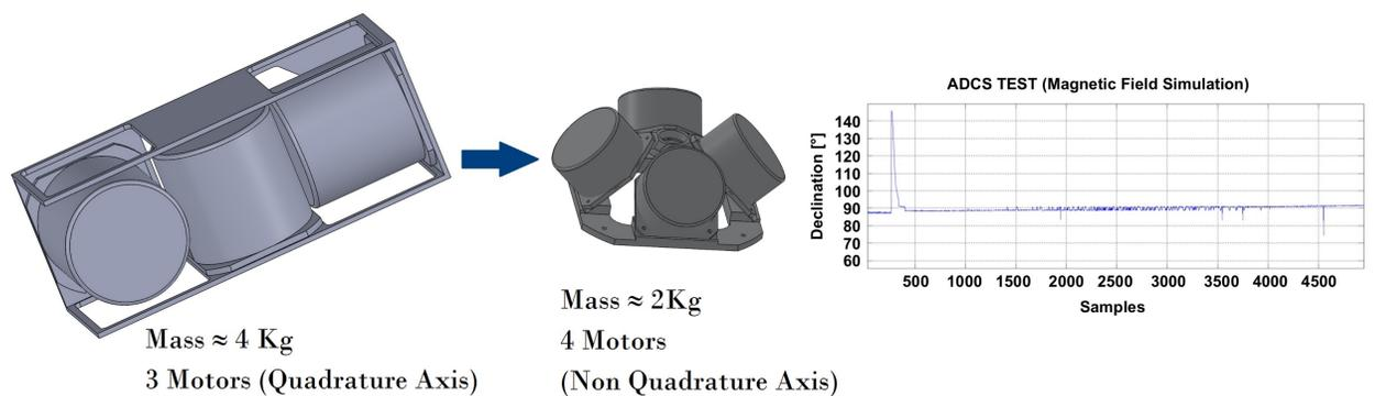
Fig. 3. Structure design configuration changes for reaction wheels module (1996 - 2016).
