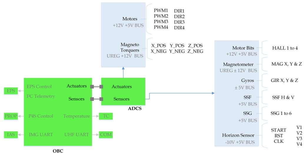
Fig. 4. Hardware signals and power distribution in the space segment block diagram.
