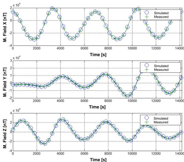
Fig. 2. Helmholtz field generator tests. Simulated and measured earth magnetic field in body reference frame. [1]
