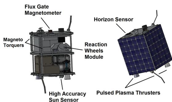
Fig. 1. Vehicle general layout. Outer and inner structure.
