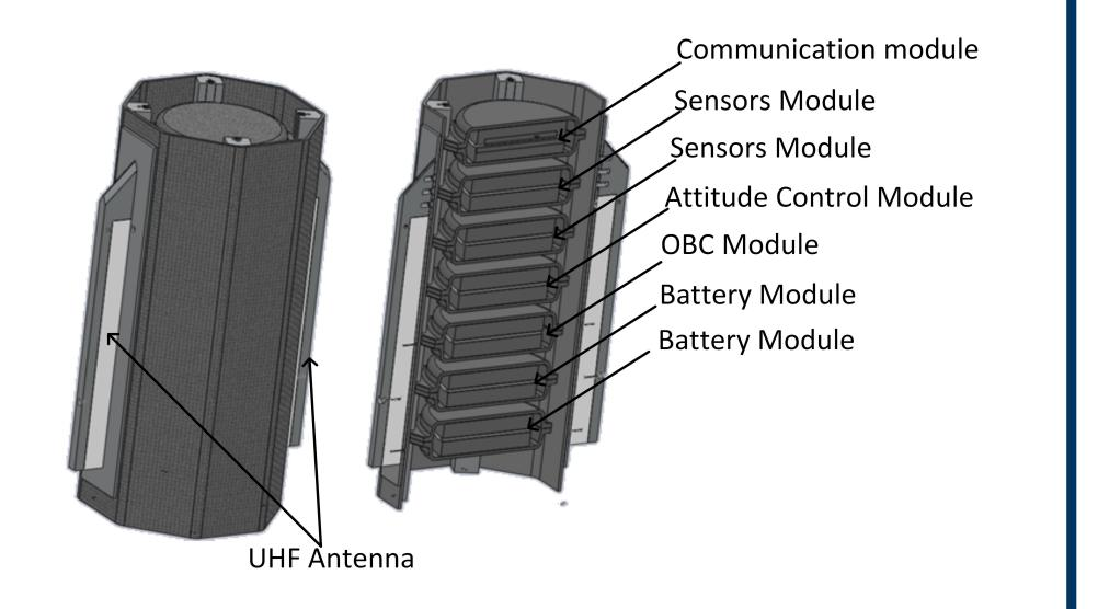
Figure 1: Structural configuration for orbital mission
