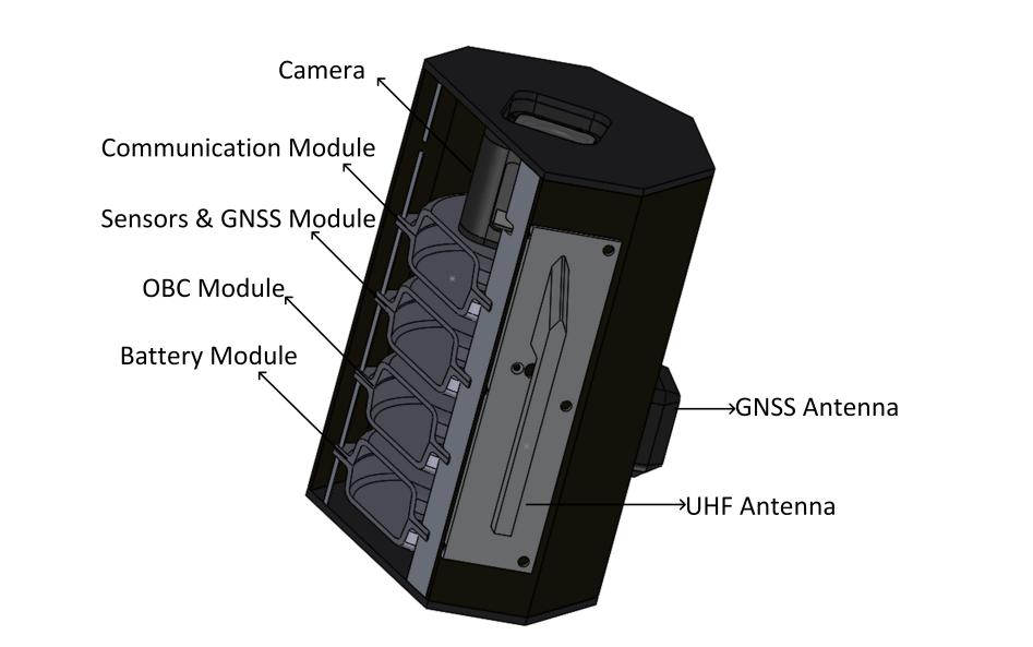
Figure 2: Structural configuration for sub-orbital mission
