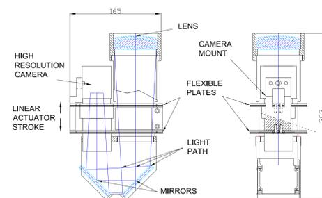
Figure 4: Focusing mechanism for high resolution camera.
