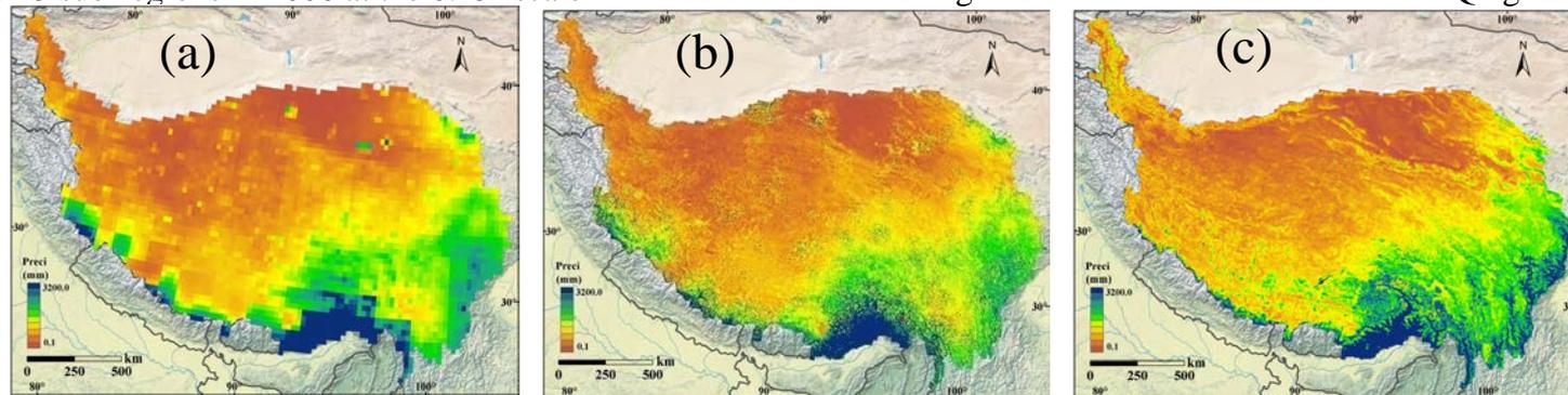
Fig. 11. (a) Accumulated monthly TMPA precipitation data for 2006 at 0.25° resolution. (b) Downscaled results based on GWR before residual correction at 1 km resolution. (c) Downscaled results based on Cubist before residual correction at 1 km resolution.
