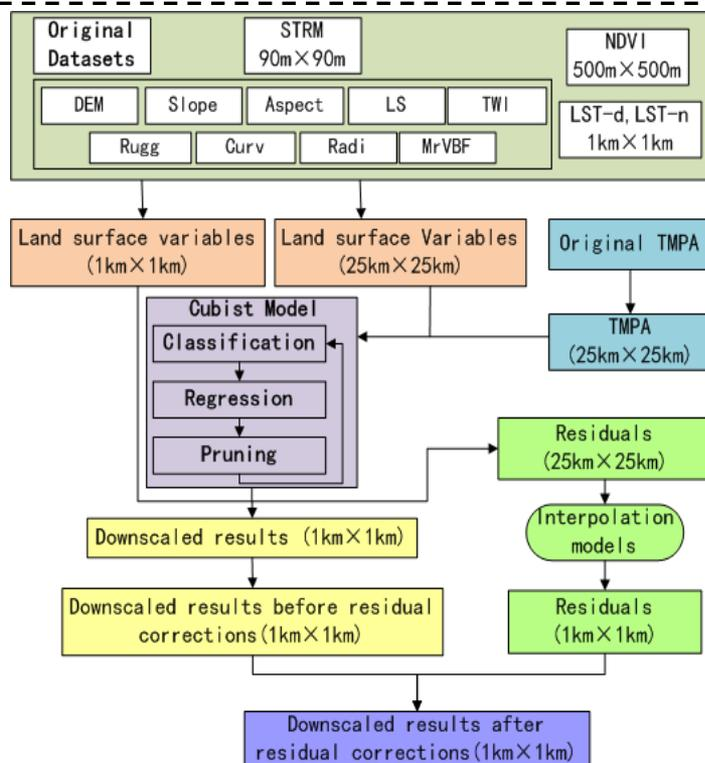
Fig. 6 Flow chart for the Cubist-based downscaling algorithm
