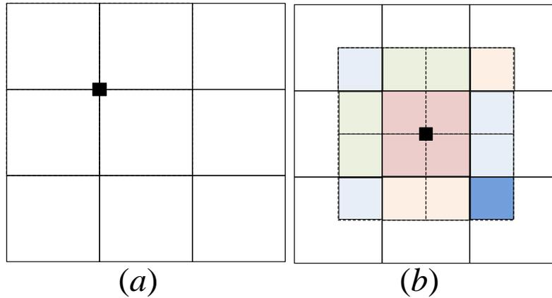
Fig. 18. The number of neighboring TMPA pixels ( $0.25^\circ$ ) was varying with the with the center of moving window located in (a) the cross of the four TMPA pixels; (b) one of the TMPA pixels.
