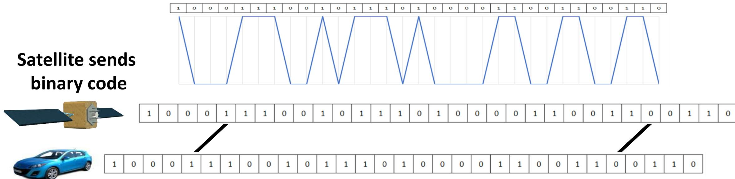
***User's receiver generates same binary code that it should be hearing from the satellite at a particular time***
