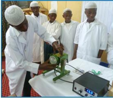
Mounting the sample on the Clinostat
