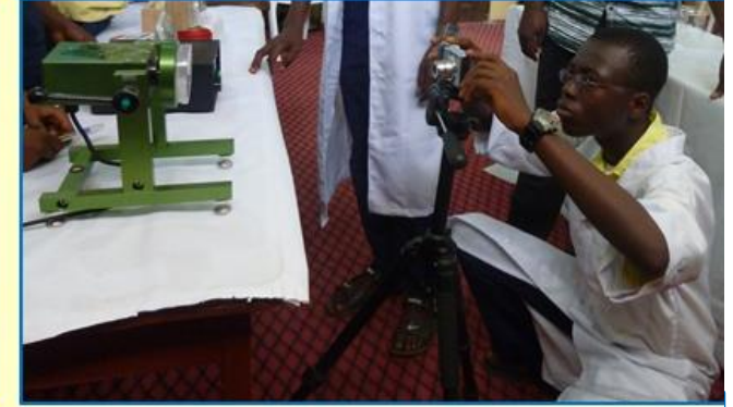
Using a digital camera to collect periodic data from the rotating clinostat
