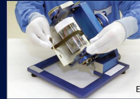
Airbus RPM 2.0 configured with experimental vessel
