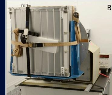
KSC Slow Rotating Clinostat in ISS stowage locker configuration
