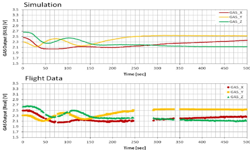
Analysis through comparison of simulation and flight data
