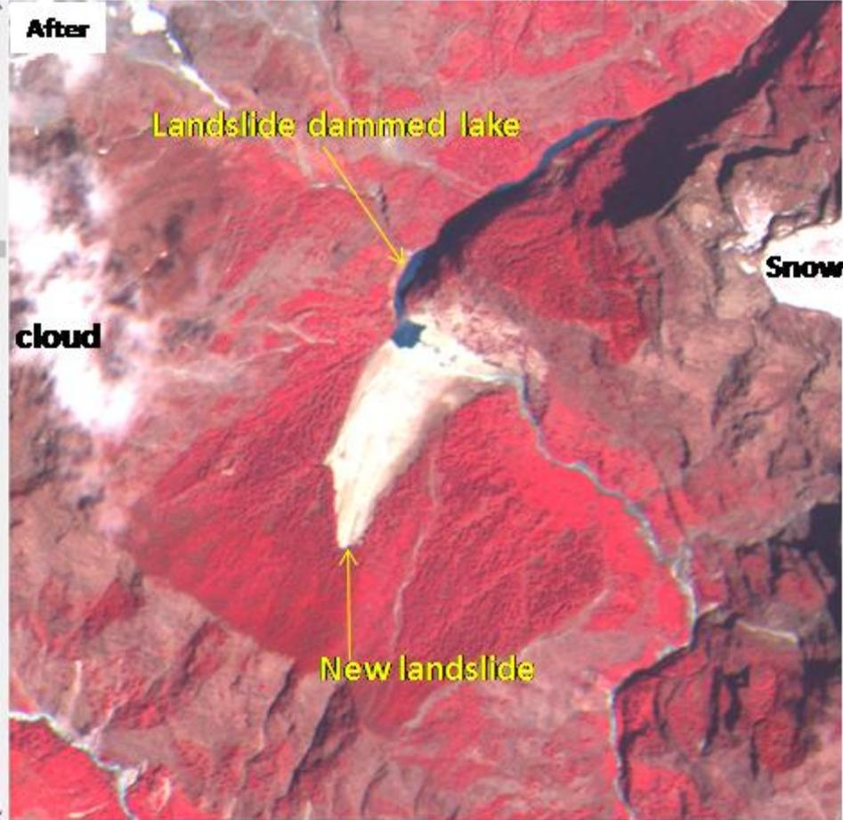
Observation: A new major landslide has blocked the valley resulting in development of a lake. Several other small new landslide are also seen.
