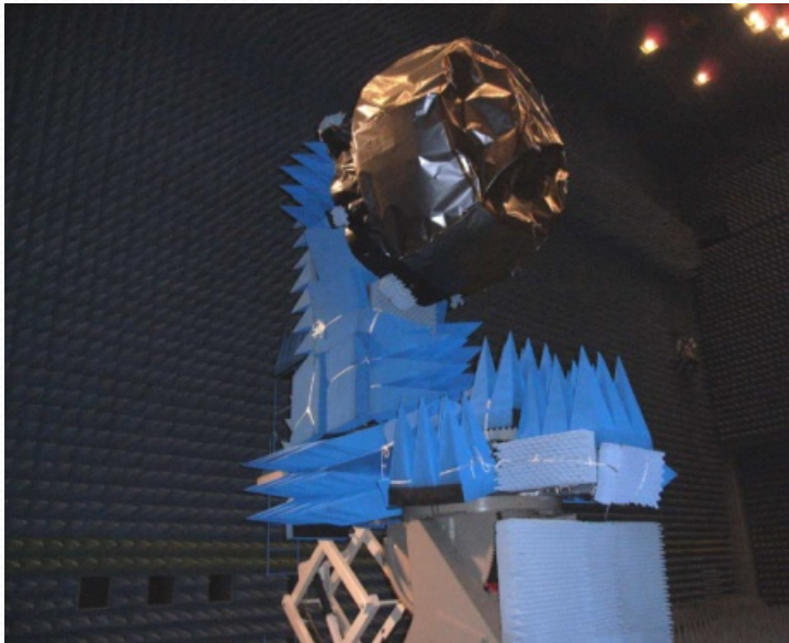
PFM L-band Antenna Pattern Test (July 2008)
