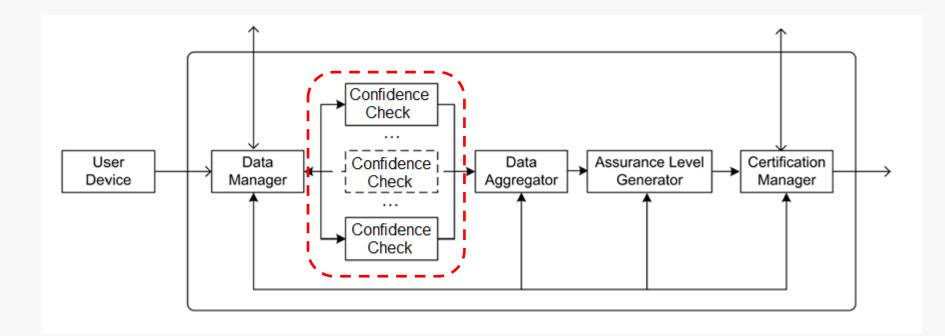
Confidence checks are algorithms that verify if signals are intact (not intentionally modified).
