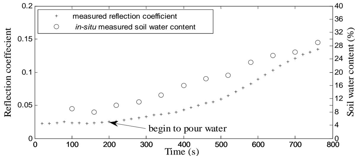
Comparison between reflection coefficient and *in-situ* measured water content
