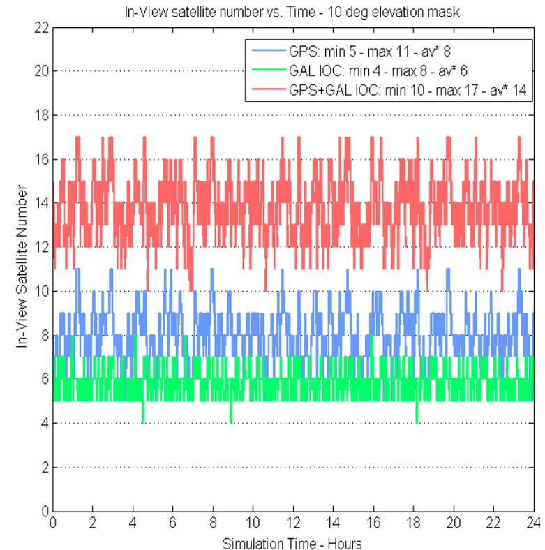
GPS and Galileo (FOC left, IOC right) visibility vs. time at LEO (817 km)
