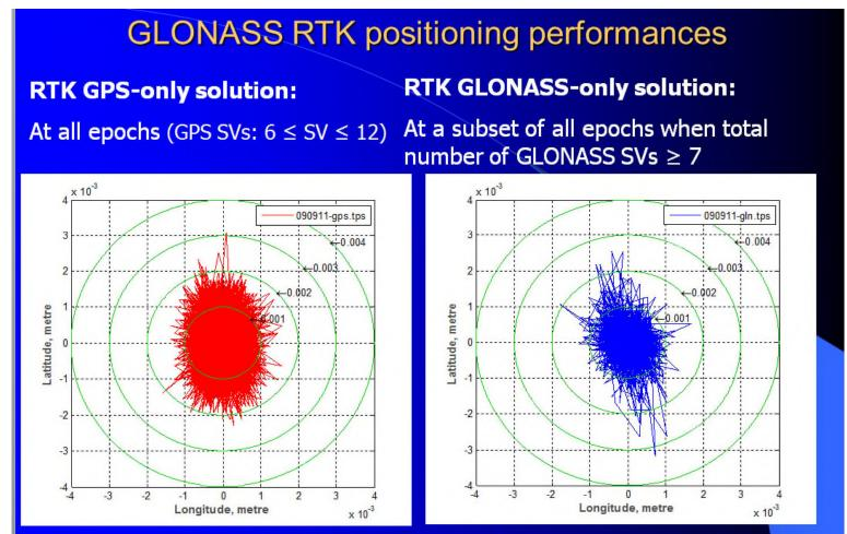
Accuracy of GLONASS RTK positioning is the same as GPS RTK accuracy provided enough number of GLONASS satellites are available for positioning.
