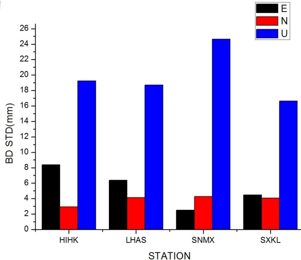
Horizontal position accuracy of CMONOC test four station is about 4-8mm
