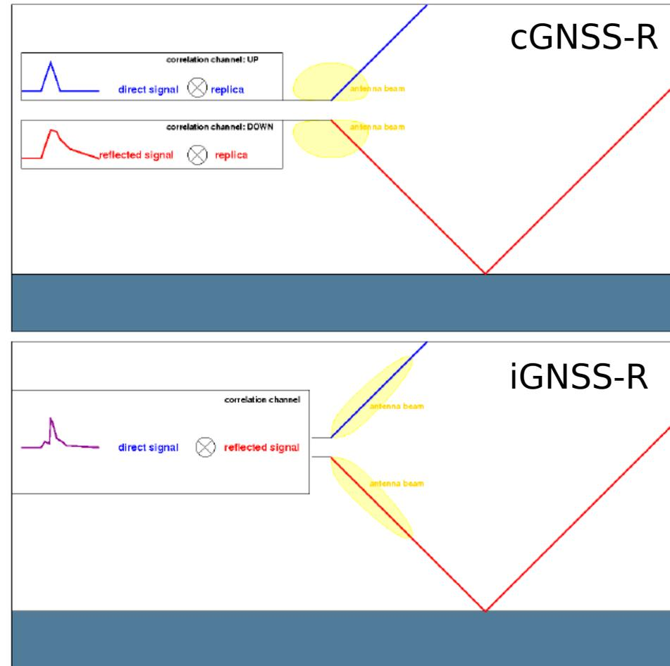
Illustration of conventional clean-replica GNSS-R (top) and interferometric GNSS-R, suggested in [Martin-Neira et al., 2011] (bottom). Figure from [Jin, Cardellach, Xie, 2014]
