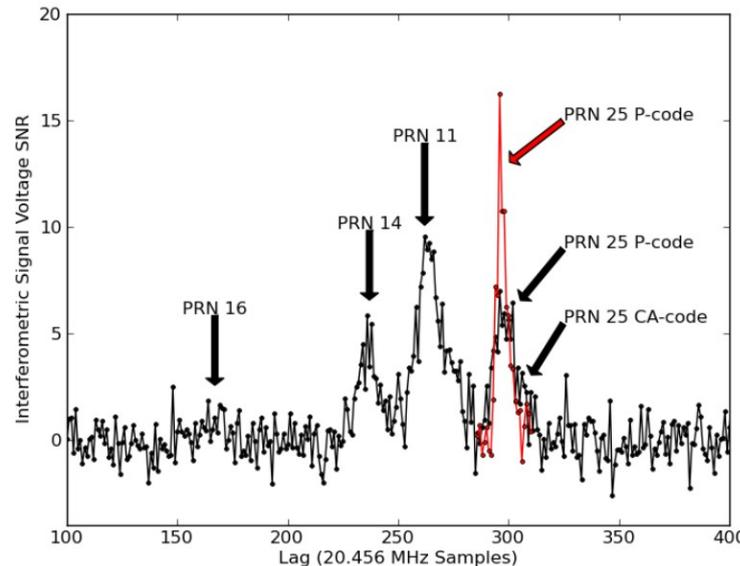
[Lowe et al., 2014] Actual airborne iGNSS-R (black) and rGNSS-R (red). From raw data obtained in 2002 flight over Pacific Ocean.
