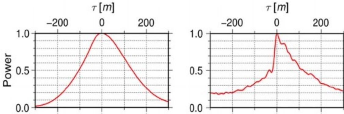
[Cardellach et al., 2013] Waveforms of open waters reflected signals (airborne, 3000 m. altitude), and the altimetric GNSS-R solution. SSH gradients of 2cm/km have been measured.
