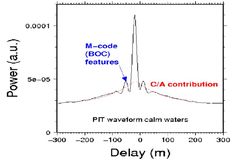
[Rius et al., 2013] Actual GNSS-R airborne data, 200 m. altitude over calm waters. IGNSS-R acquisition technique.
