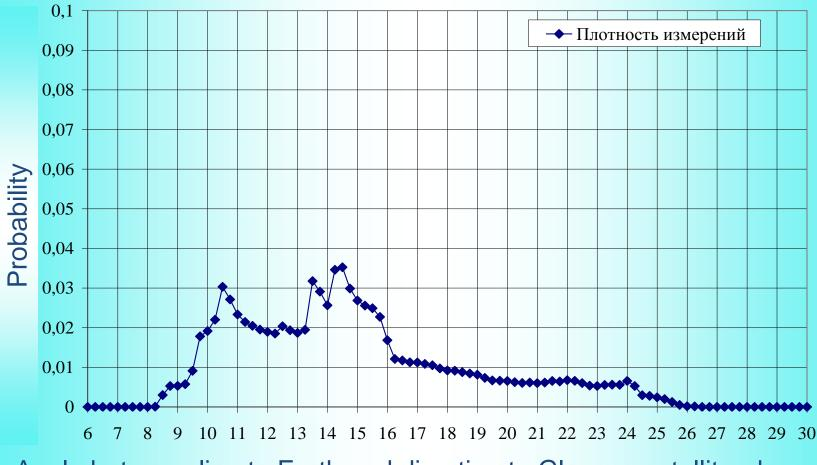
Angle between line to Earth and direction to Glonass satellite, degree
