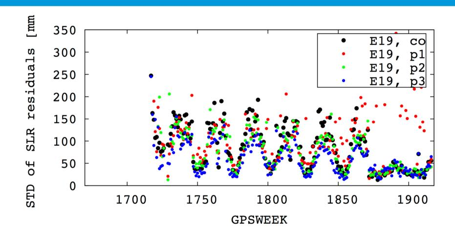
The SLR residuals are confirming the overall orbit accuracy (3D – 1 Sigma) of 10 – 20 cm Notice improvement thanks to improved modelling starting week 1873
