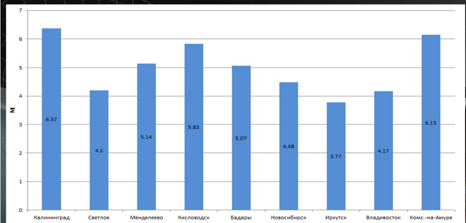
Differential corrections for standard parameters of upgrading from SC-42 to PZ-90.11 for different sites vary in the range of up to 6-7 m
