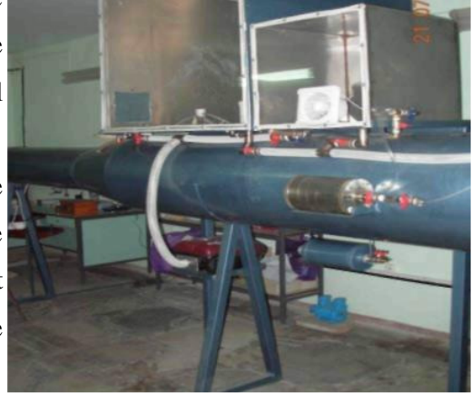
Fig. 8. The aerodynamic (fragment) tube with data acquisition system.
