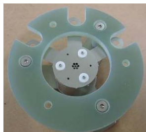
Fig. 7 Laboratory model of carbon nanotube cathode.
