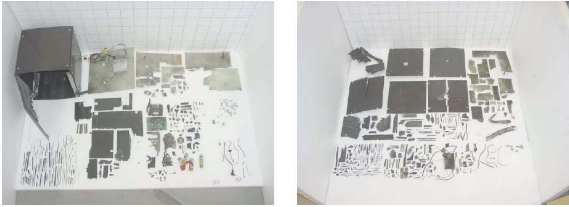
Fig.-3 Major fragments generated in impact tests
