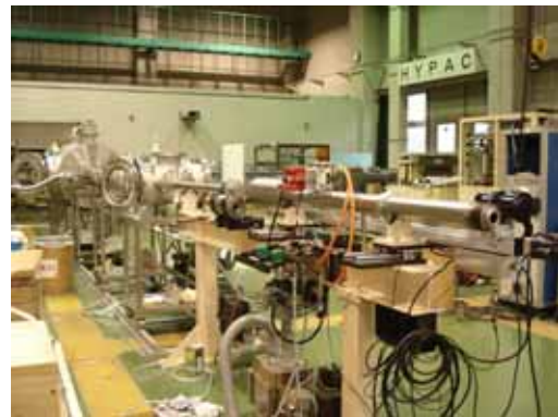
Fig.6 Newly introduced two-stage gas gun at Sagami-hara Campus of JAXA.
