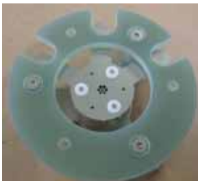
Fig. 7 Laboratory model of carbon nanotube cathode.
