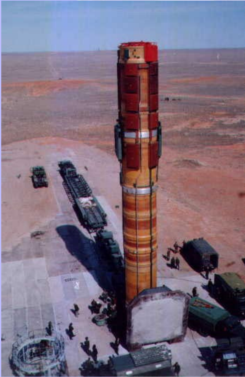
R-36M missile installation into a silo launcher
