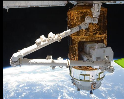
EP with unpressurized cargo transferred by SSRMS
