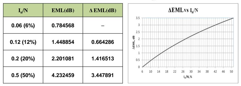
The degraded link energy margin  $\Delta$ EML (dB) value reflects energy margin loss compared to the case of single entry interference 6%. The  $\Delta$ EML (dB) will not exceed 0.66 – 3.45 dB corresponding to the typically available energy margin in the current FSS networks.
