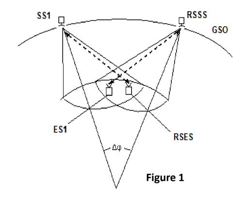
On Figure 1: SS1 – space station of the assessed system ES1 – earth station of the assessed system RSSS – space station of reference system RSES – earth station of reference system
