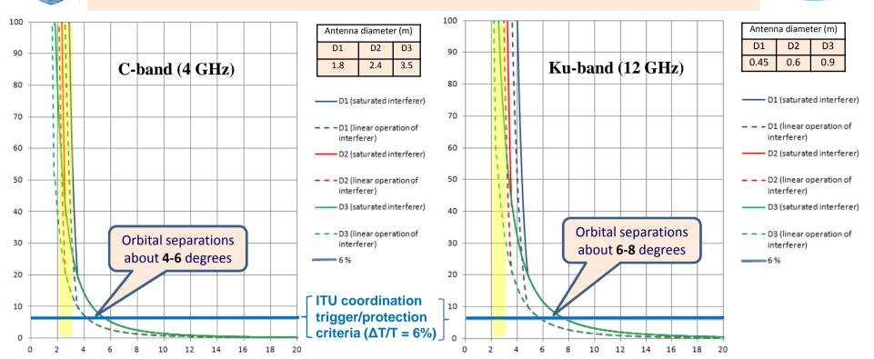
The resulting  $\Delta T/T > 6\%$  in **C-band** for orbital separations less than about **4-6 degrees.**
