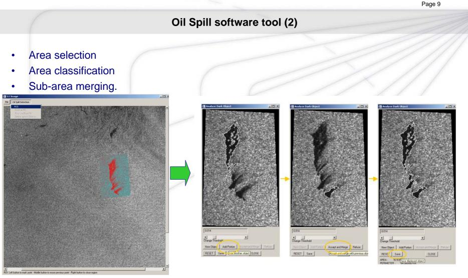
The oil spill classification is performed by means of use of neural network properly trained.
