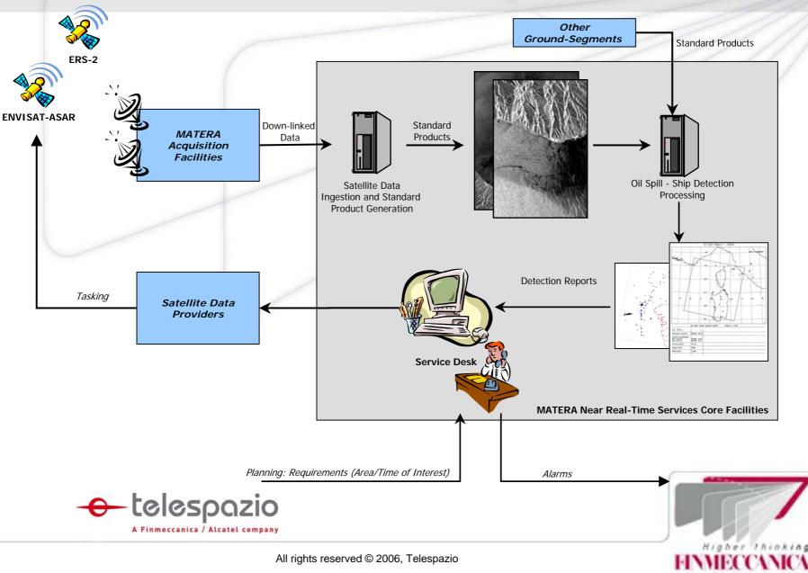
The monitoring is based on the repetitive observation performed by Remote Sensing satellites.
