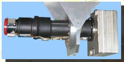
Multispectral camera (4 ranges) (weight = 18.7 kg)
