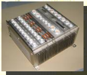
On-board information system unit (weight = 13.3 kg)
