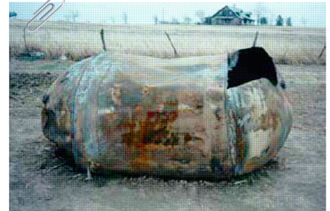
Delta II second stage propellant tank found in Texas, 1996
