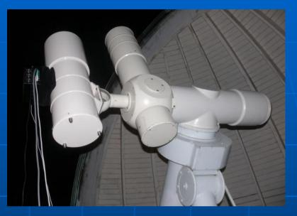
The subsystem is based on 22-cm class instruments with FOV up to 4.8°
