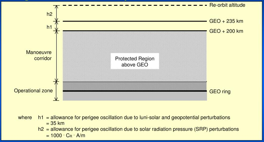
The IADC and other studies have found that fulfilling the additional condition at the end of the disposal phase would give an orbit that remains above the GEO protected region: the eccentricity should be less than or equal to 0.003.
