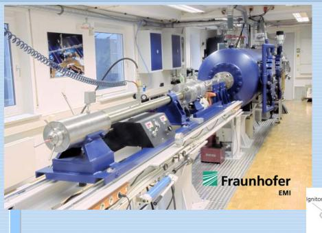
Launch Tube dia. ranging from 6.5 mm to 15 mm.
