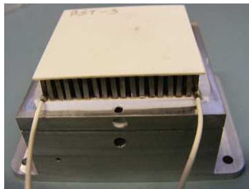
Bismuth Telluride Boron Carbide Composite Based Thermoelectric Materials and Modules (University of Leicester)
