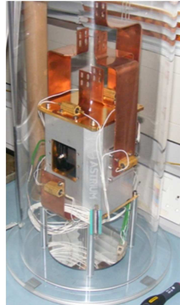
Electrically Heated 5 W RTG Laboratory Prototype (University of Leicester)
