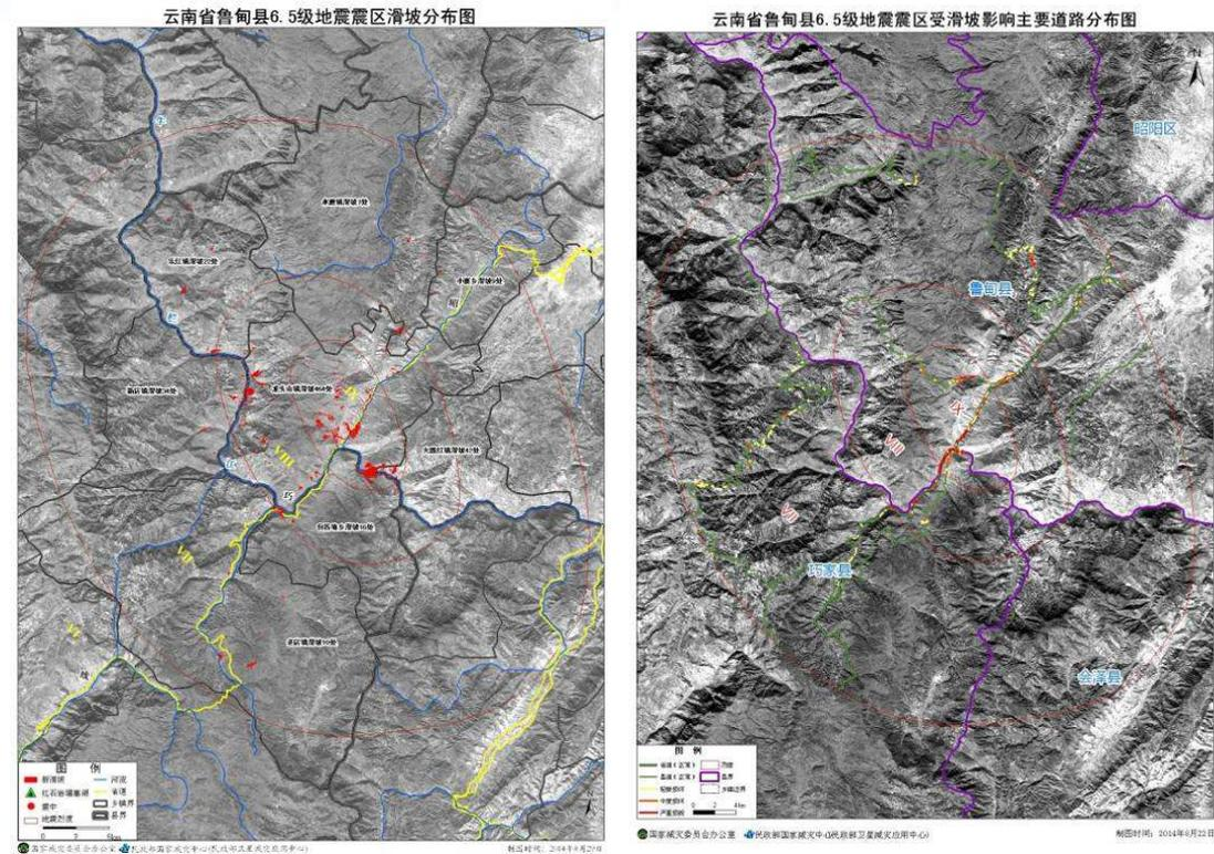
Fig 11 Landslides and their impacts on traffic lines
