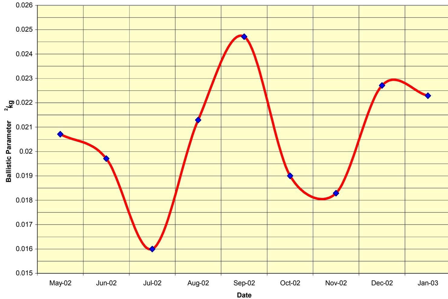
**Fig. 1 – Ballistic parameter evolution (monthly averages) after the BeppoSAX deactivation (May 2002 – January 2003)**
