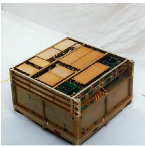
Figure 2 Imager tray with power and communication trays stacked on it.
