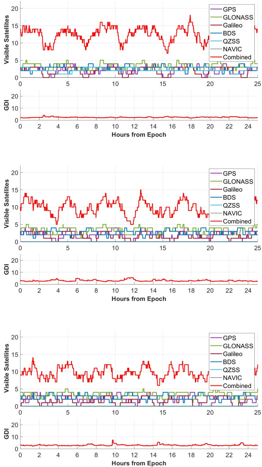
Figure C9. L5/L3/E5a/B2 visibility for GEO at 180 deg, 240 deg and 300 deg
