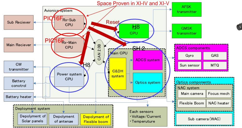
Combination of "High performance but not space-proven" processor and "Low performance but space-proven" processor
