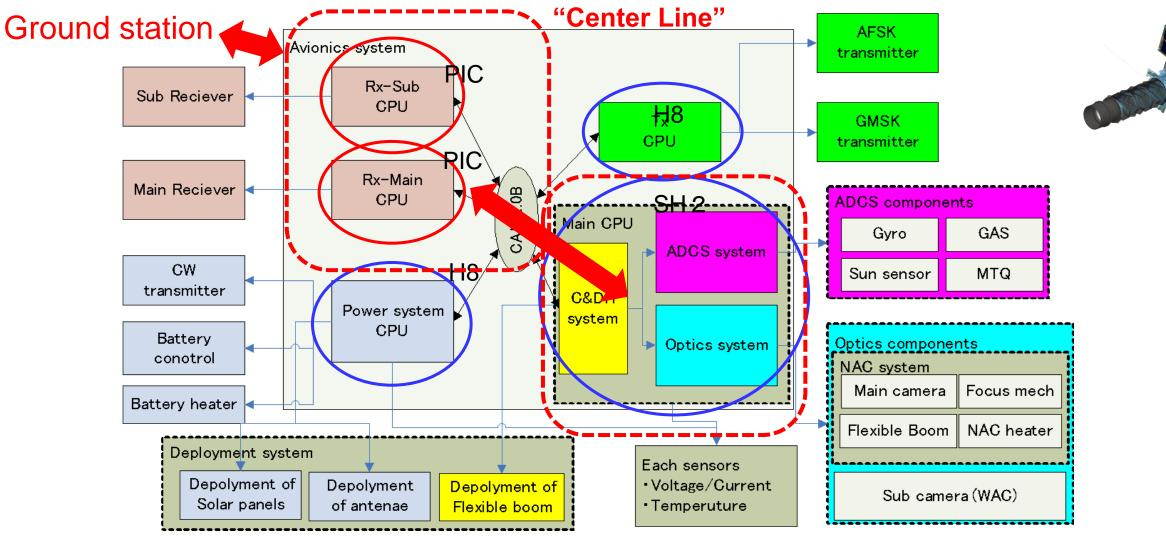
Combination of "High performance but not space-proven" processor and "Low performance but space-proven" processor
