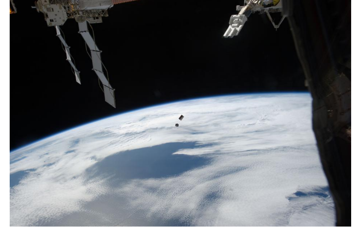
First CubeSats deployment from the ISS. © JAXA
