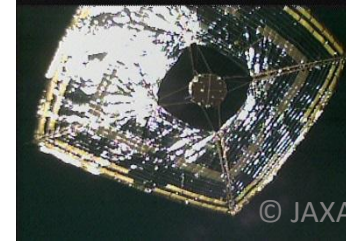
IKAROS (2007-2010): 315kg World's first interplanetary solar sail
